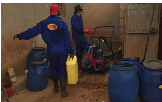
Figure 1: The eVac can be wheeled or carried to any pit location
