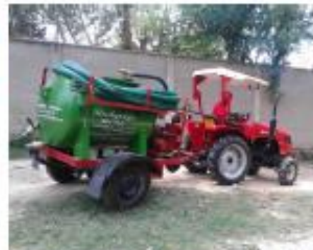
Figure 4: Developed means of Emptying & Transporting Faecal Sludge
