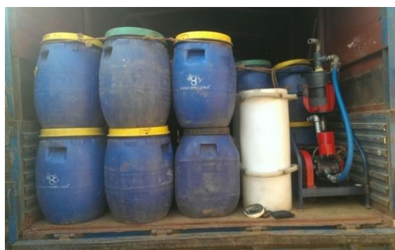
Figure 2 eVac with sludge barrels in Pit Vidura truck
