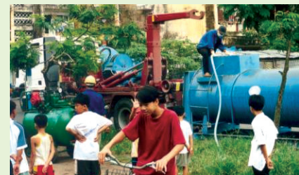
Photo 10: Intermediate storage tank located in the nearest accessible road. (Sandec, 2002, Hai Phong, Vietnam)
