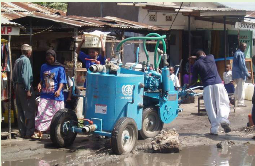
Photo 8: This Vacutug mini-tanker manufactured in Bangladesh, under the supervision of Manus Coffey and Associates, is used in a UN-Habitat co-financed waste management project. (UN-Habitat, 2003)
