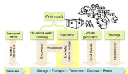
Figure 1: This module centres mainly on the management of faecal sludge from its source to its final disposal or reuse.
