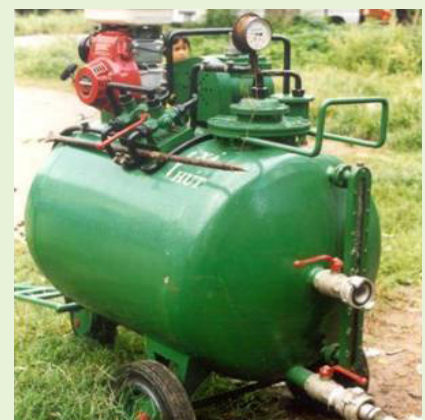
Photo 9: Mini-vacuum tug for narrow lanes. (Sandec, 2002, Hai Phong, Vietnam)
