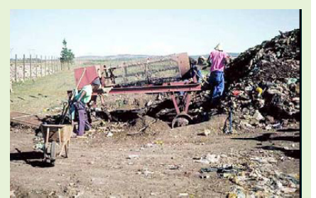
Photo 12: Sieving matured compost in a rotary sieve at Rini/Grahamstown (South Africa) co-composting works. (Strauss et al. 2003b)
