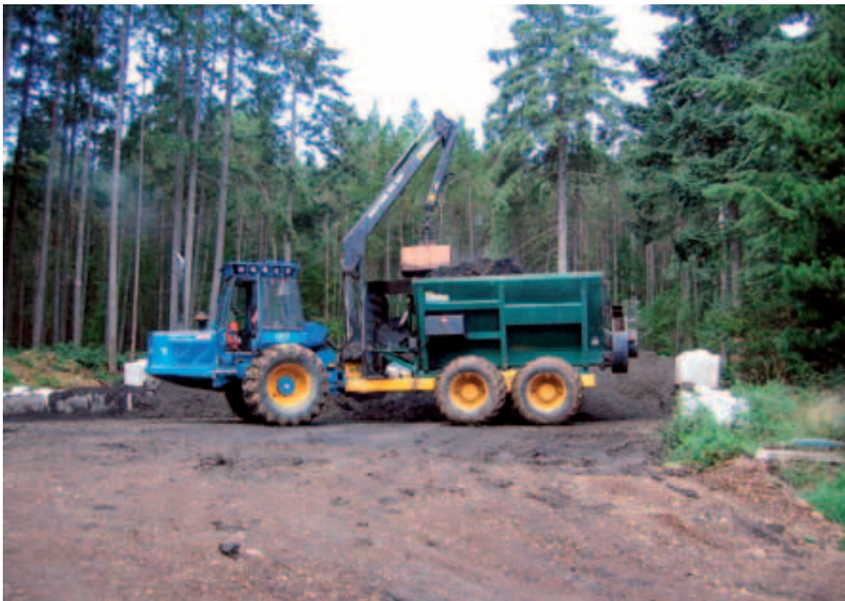
Photograph 2: A side-discharge fan applicator for forest application of biosolids. Photo © SYLVIS Environmental
