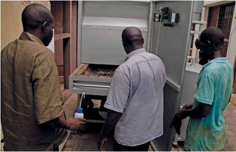
Figure 10.11 FaME (Faecal Management Enterprises) project pilot scale kiln for combustion of faecal sludge to heat oil in industrial processes, Thies Polytechnical University, Senegal (photo: Linda Strande).
