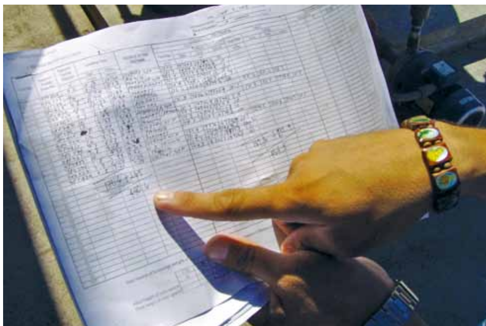
Figure 11.5 Reception reports track the total number of loads delivered, the time, date and driver's name. These records are important to maintain for all faecal sludge treatment plants (photo: David Robbins).
