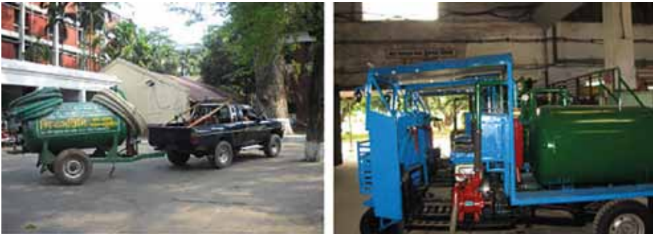
Figure 4.11 The Mark III (left) and Mark IV (right) models of the BREVAC collection and transport device (photo: Peter Edwards).
