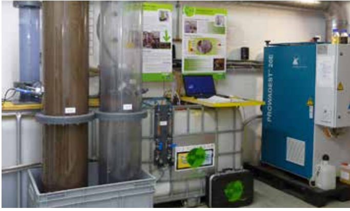
Figure 2: Combined nitrification and evaporation set-up at Eawag enabling complete nutrient recovery from urine (the South African nitrification and evaporation reactors are similar).
