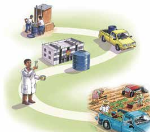
Fig. 1: Schematic drawing of urine collection and processing into fertiliser in the brochure used to explain the VUNA project to toilet users.
