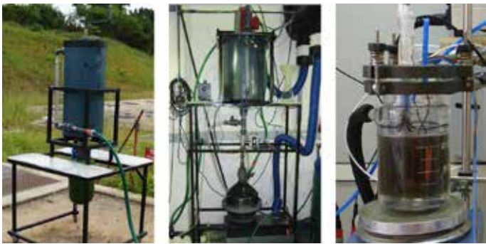
Figure 3: Left: Manually operated struvite field reactor at the Newlands-Mashu field test site in eThekweni; Centre: Fully automated struvite reactor at the PRG laboratory; Right: Electrolysis cell for urine treatment at the Eawag laboratory.
