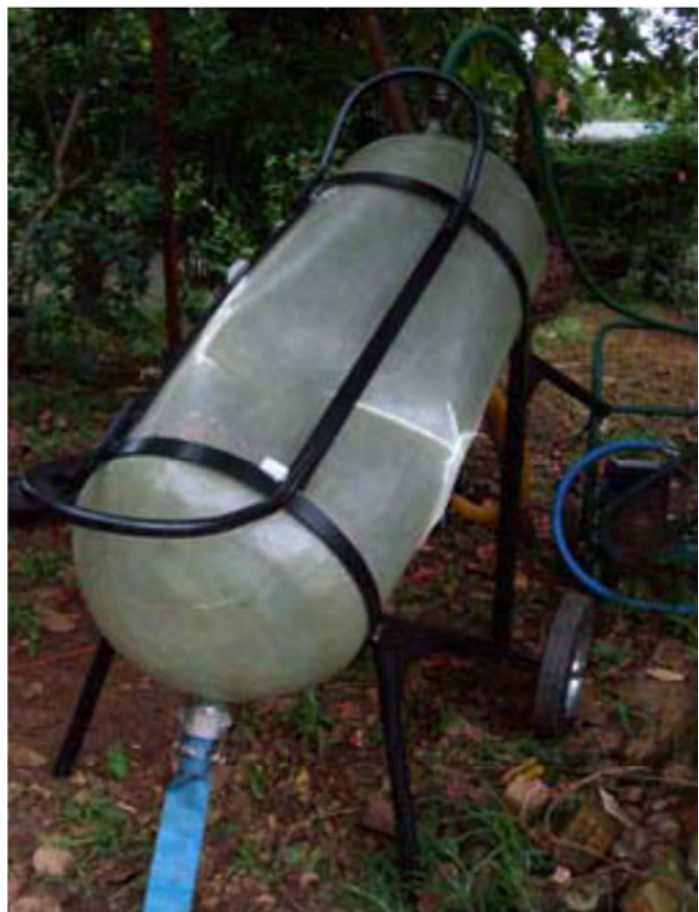
Figure 7.4 A custom made 180 litre fibreglass tank which imploded under vacuum pressure
