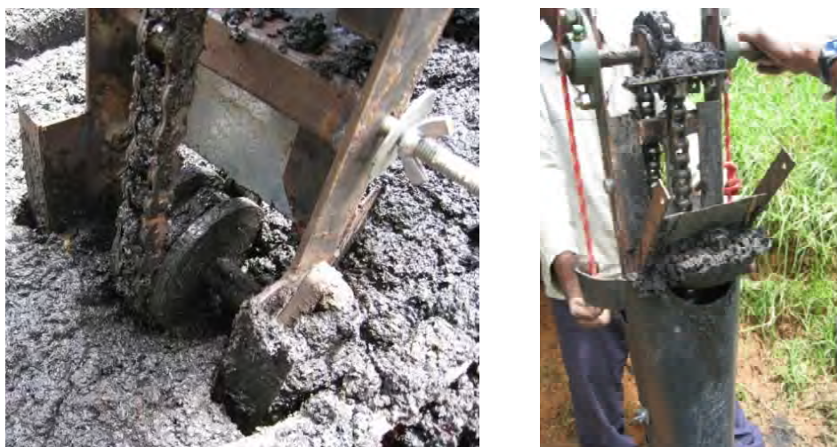
Figure 3.3 Second prototype of Gobbler with single chain and sprung scraper
