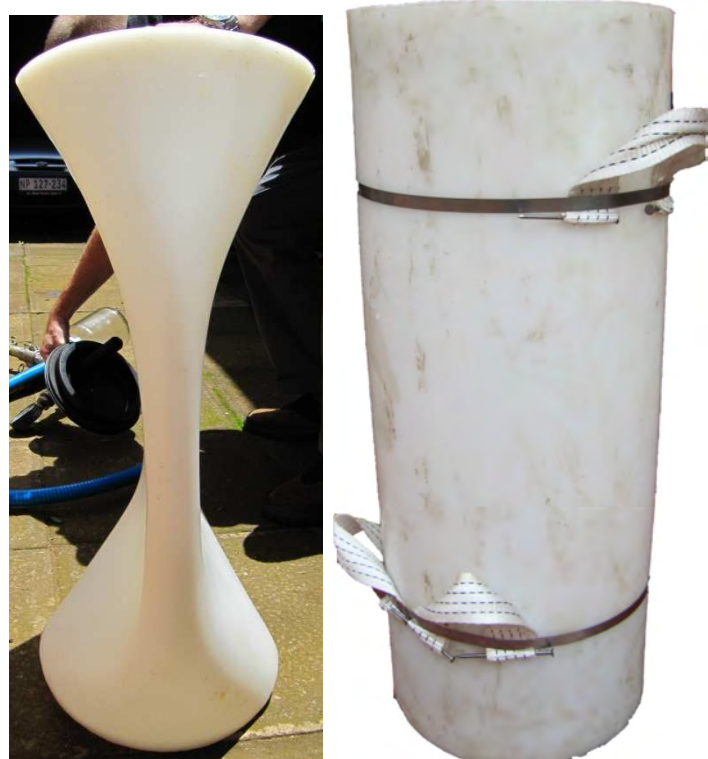
Figure 7.6 7 mm thick vessel imploded under vacuum (left) and 14 mm thick vessel currently in use with carrying straps (right)
