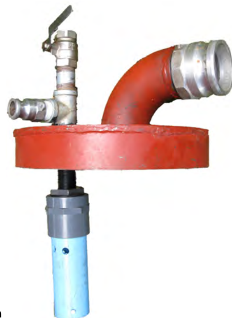
Figure 7.7 The sludge hose collapsed near the point of connection during testing (left); the “suck only” lid with steel elbow for connection to sludge hose (right)
