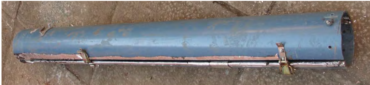
Figure 4.3 Hinged sleeve enables blockages to be more easily removed
