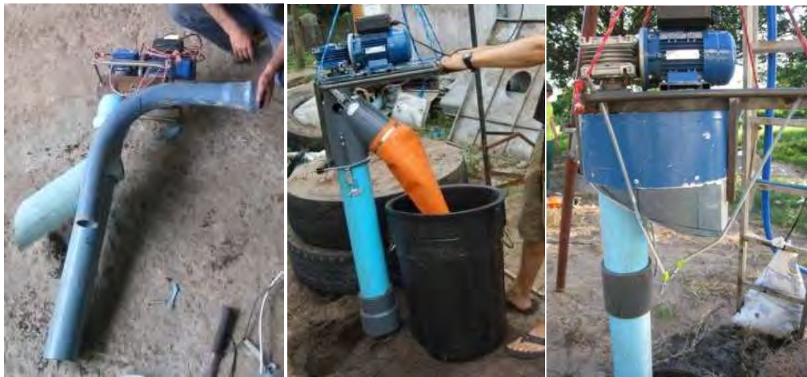
Figure 4.5 Swept elbow termination compared with 45 degree tee termination (left), 45 degree tee with lay flat hose (centre) and 45 degree plate termination (right).
