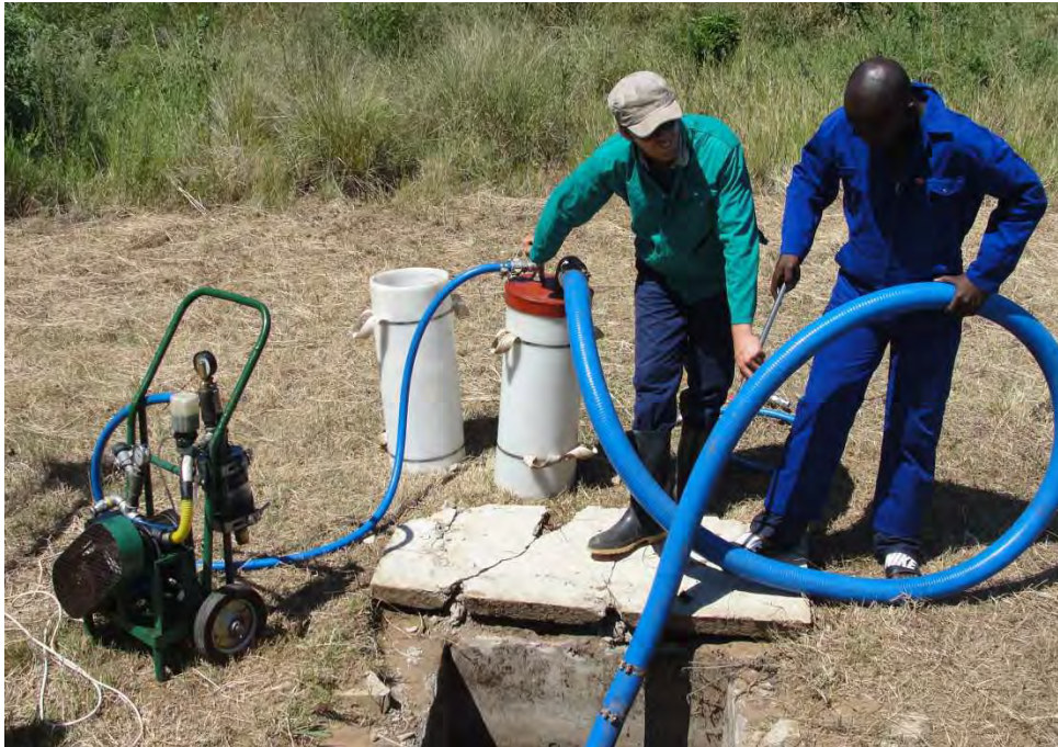
Figure 7.10 eVac emptying a pit using multiple pressure vessels with carrying handles
