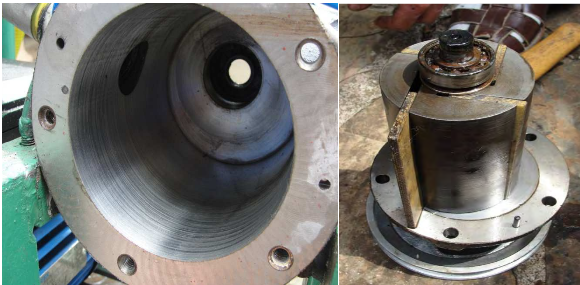
Figure 7.2 The components of the vane pump (the stator on the left, and rotor with removable vanes on the right)
