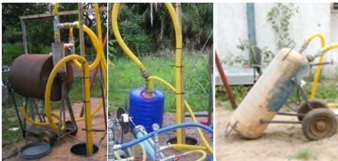
Figure 6.8 Various containers trialled as vacuum tanks: steel drum (left); Hippo Roller (centre) and gas canister (right)
