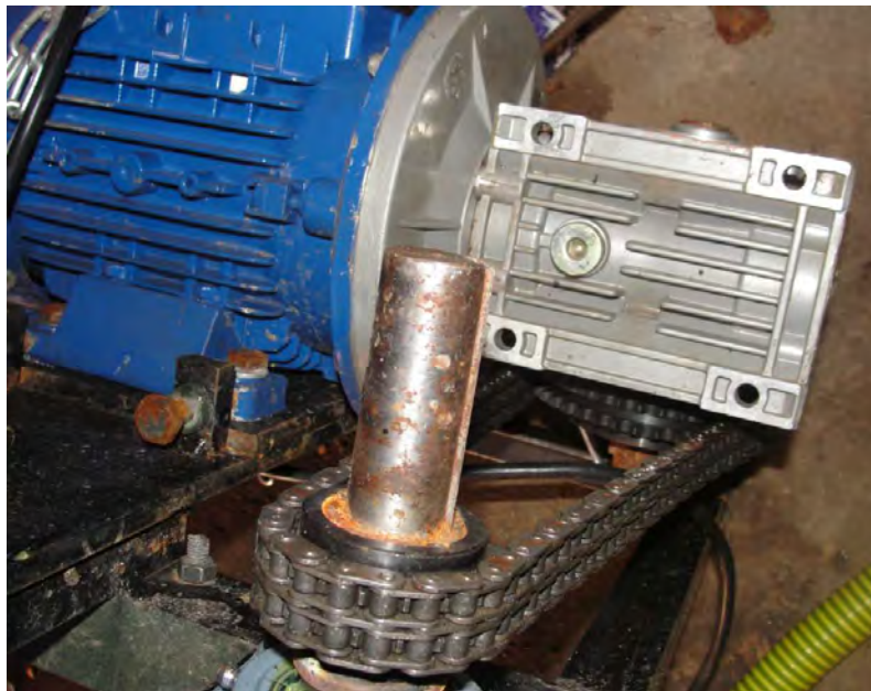
Figure 4.2 Offset gear box with chain and sprockets
