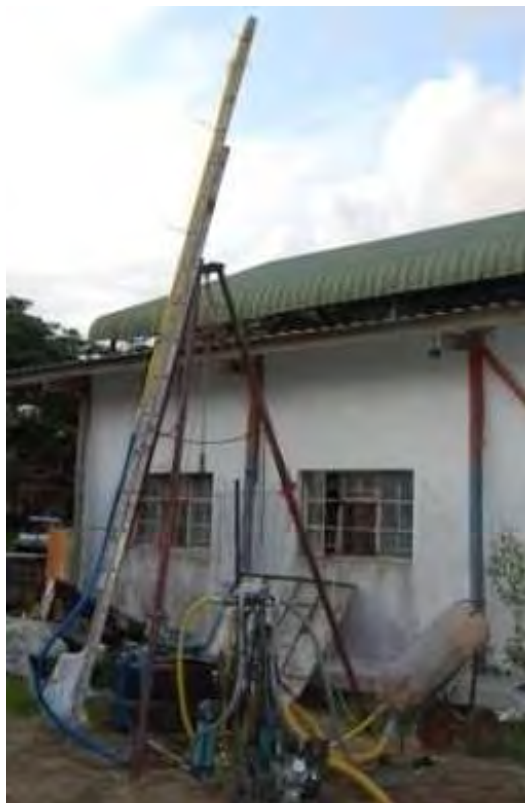
Figure 6.7 Testing the capacity of the Nano Vac to pump vertically
