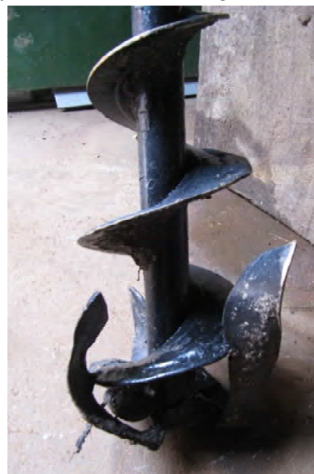
Figure 4.4 Blades added to auger point
