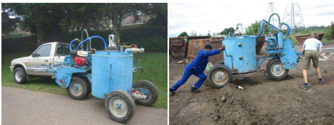
Figure 5.10 The size of the Vacutug compared to 1 ton bakkie (left) and the Vacutug unable to power itself over a small earth ridge (right).
