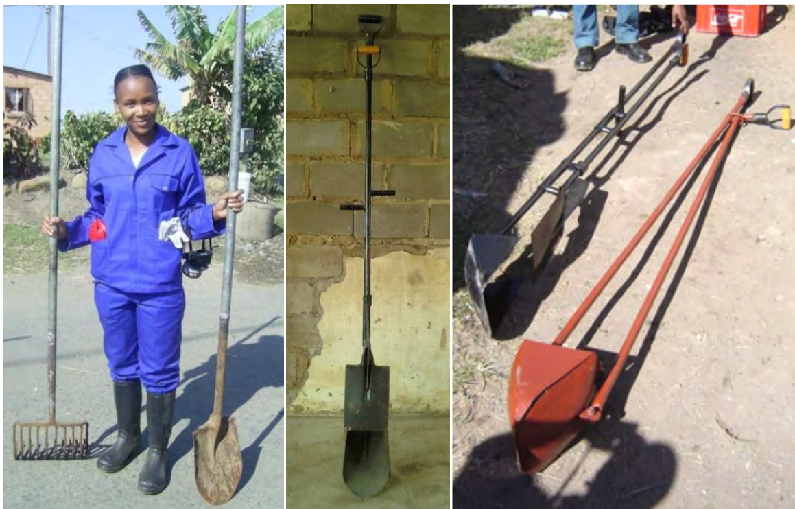
Figure 1.3 Tools used for manual pit emptying at eThekweni
