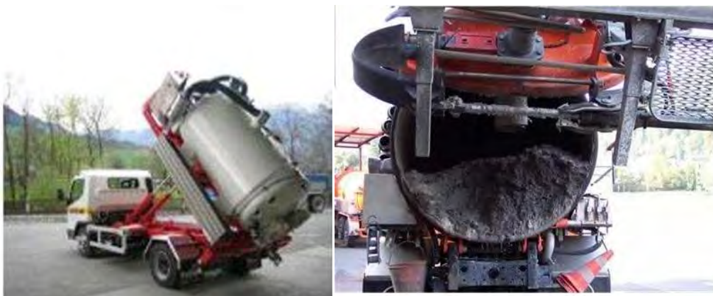
Figure 5.9 A solid liquid separation machine (Eawag and Sandec)
