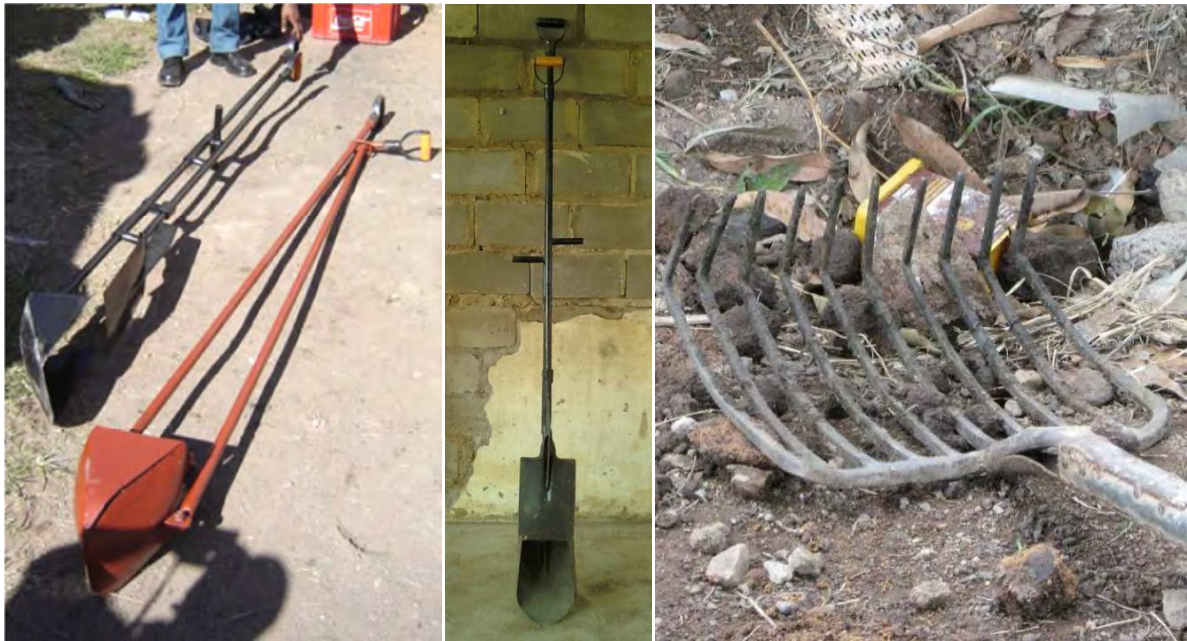
Figure 4.8 Some of the hand tools developed and tested in eThekweni's pit emptying programme. The simpler tools such as long handled forks and spades proved to be more practical. The long handled grab tool pictured above left and centre was too heavy and unwieldy to be popular.
