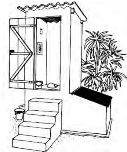
Figure 12: An eco-toilet with solar-heated processing chamber
