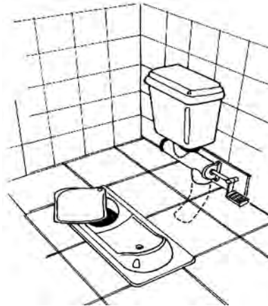
Figure 14: A mechanical, pedal-operated, ash dispenser used for school toilets in China
