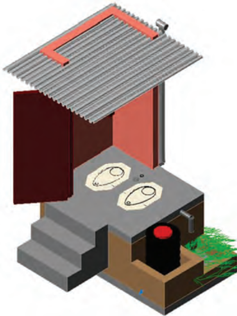
Brick work and PCC work for chamber
