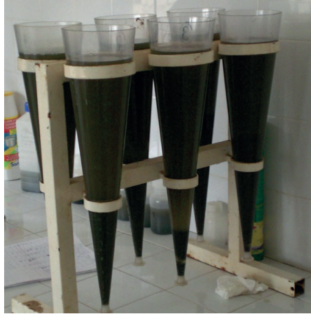
Figure 6.4 Imhoff cones being used in analyses of sludge volume index (photo: SANDEC).
