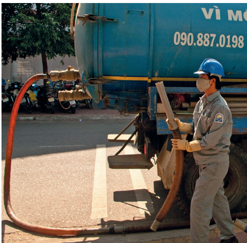
Figure 4.12 Example of correct method where the hose is easy and quick to assemble (photo: Linda Strande).
