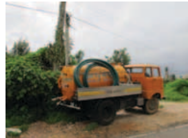
Septage is delivered to Da Lat WWTP for co-treatment with wastewater
