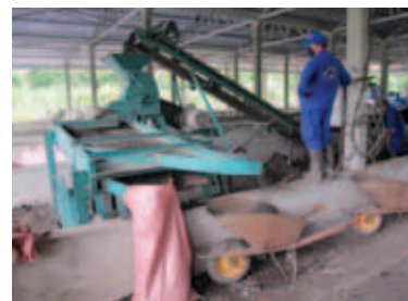
Composting of dried sludge for fertilizer production at Da Lat WWTP
