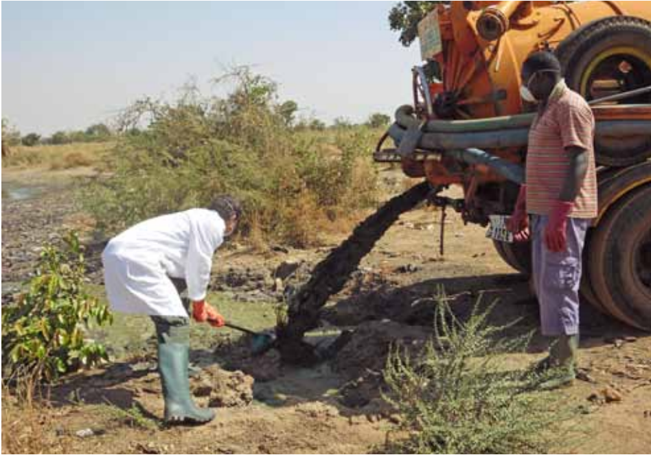
Figure 2.4 Sampling campaign to quantify and characterise faecal sludge in Ouagadougou, Burkina Faso for the design of a new faecal sludge treatment plant. Currently, none exist in the city and the only option for collection and transport companies is direct discharge (photo: Hanspeter Zoellig).
