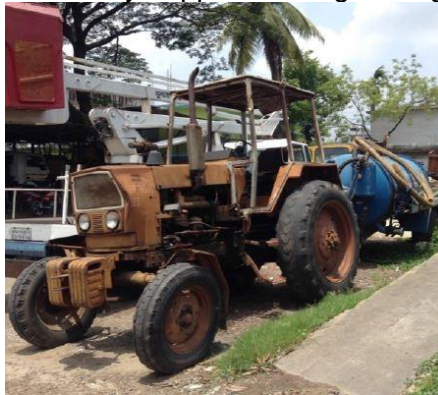
Figure 2: Tank with vacuum pump towed by tractor for faecal sludge collection (Credit: Arief Gunawan)
