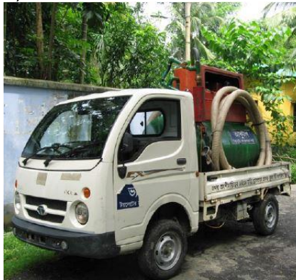
Figure 3: Vacutug for faecal sludge collection (Credit: Arief Gunawan)
