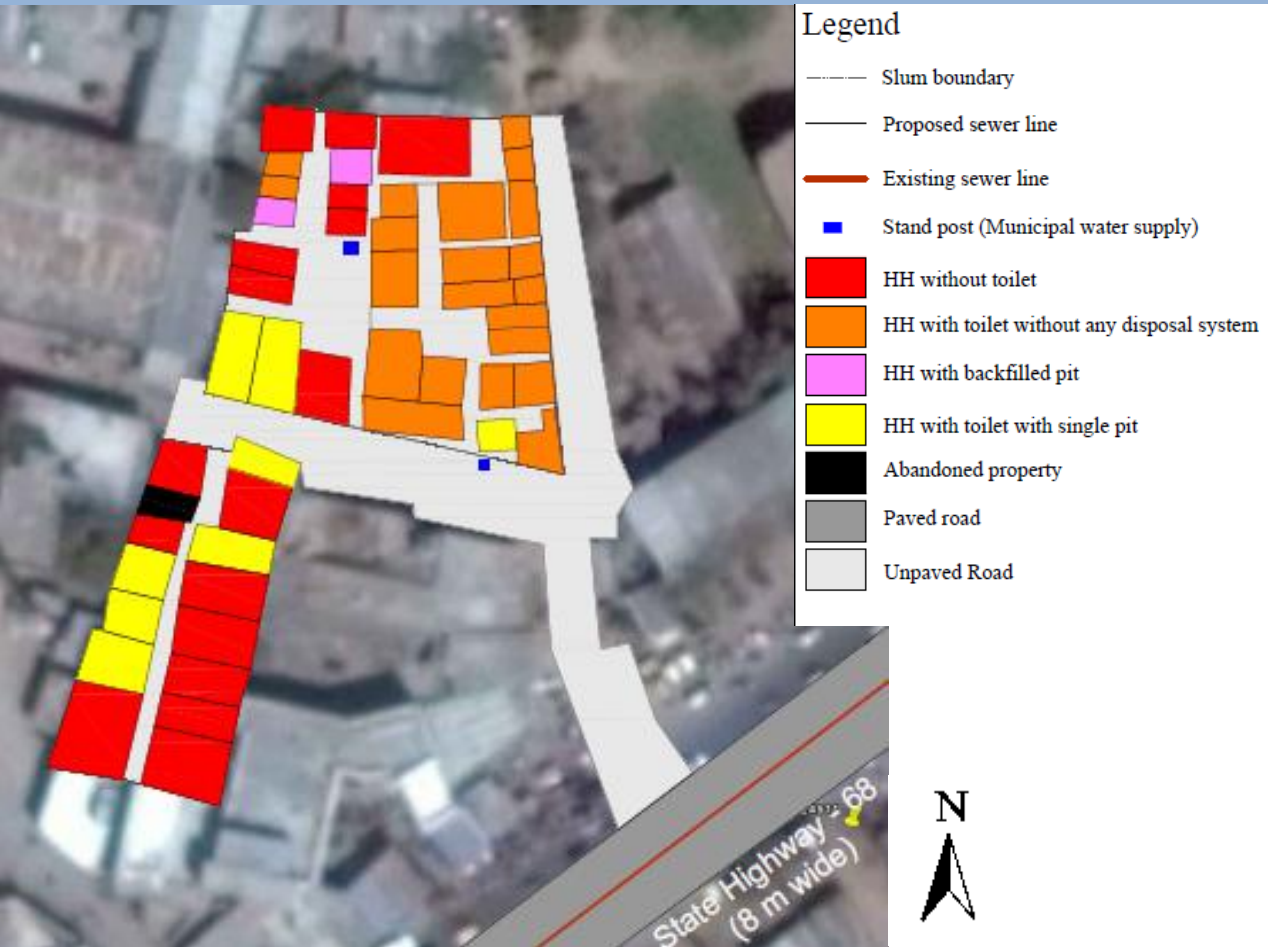
Individual toilets lack connection to disposal system
