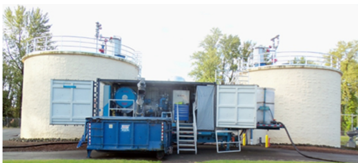
Figure 1. Trailer-mounted rotary fan press dewatering system
