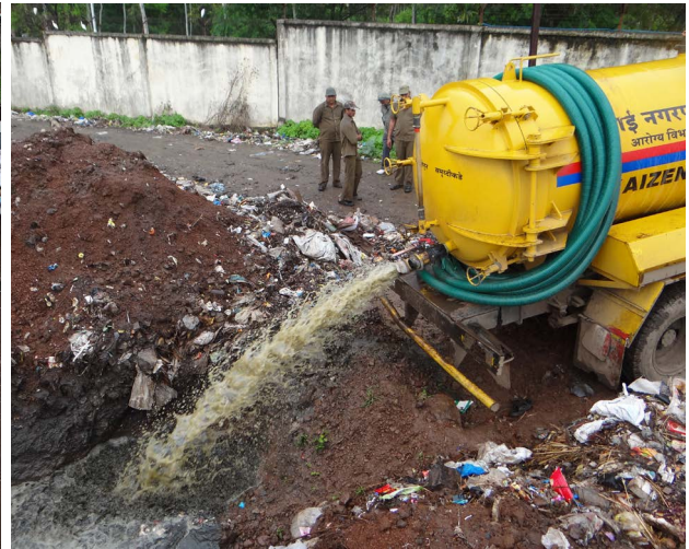
On site sanitation (toilets with septic tanks- requiring suction emptier trucks) is the predominant mode of sanitation. However very little attention is paid to
