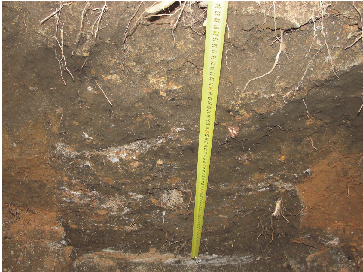
Figure 3.40 Appearance of sludge 38 months after entrenchment
