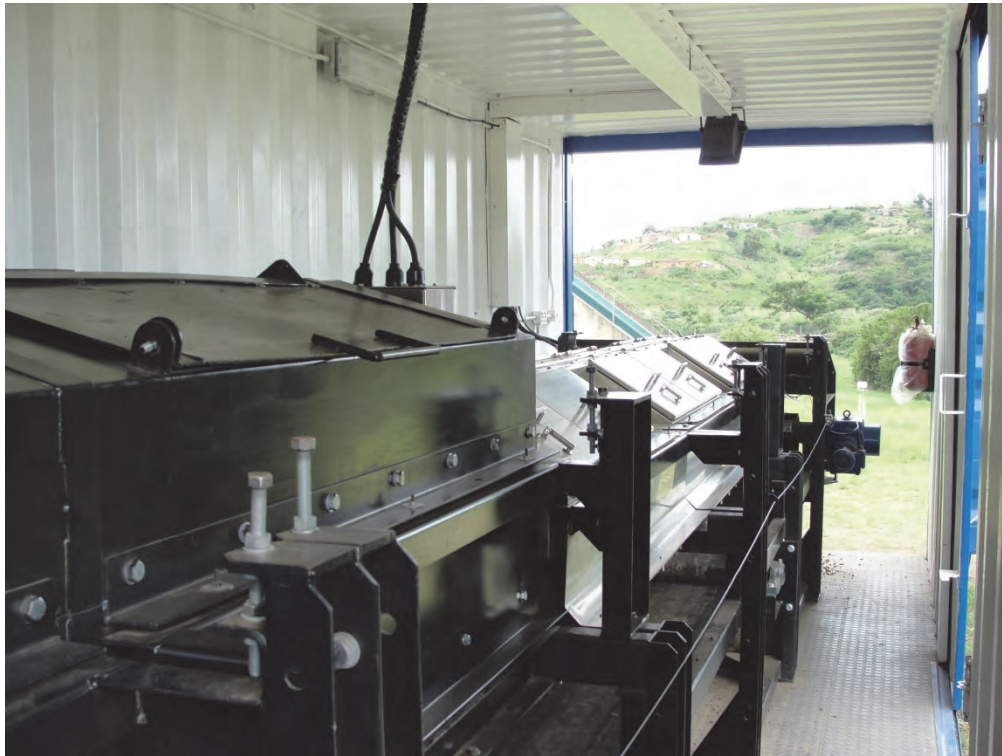
Figure 7.5 A view of the second and third stages of eThekweni's pilot LaDePa machine
