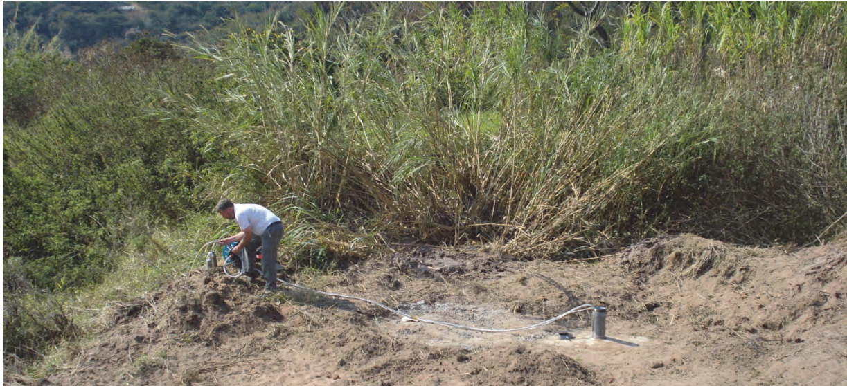
Figure 2 Sampling water from one of the monitoring wells at the Sappi site.
