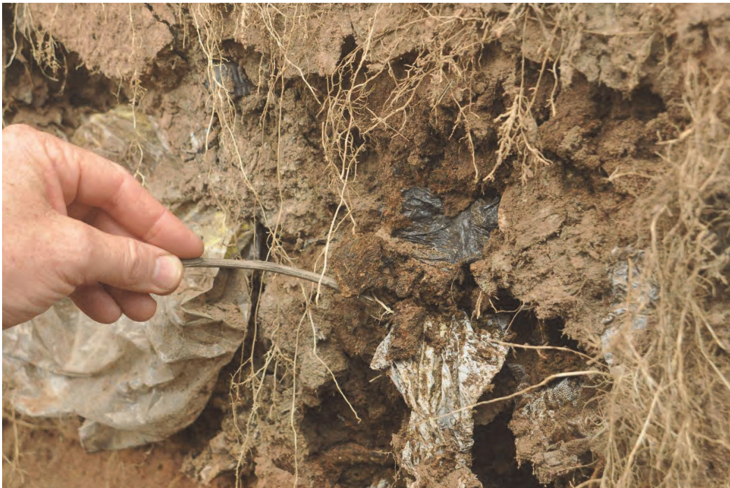
Figure 1 After four years' burial the sludge is hard to distinguish from the surrounding soil (the plastic is a good clue)
