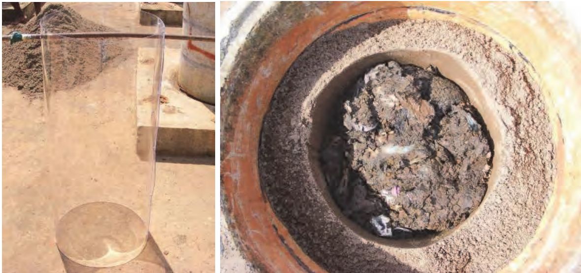
Figure 3.5 A polycarbonate cylinder (left) was used to fill the tower with a core of sludge ringed by river sand (right)
