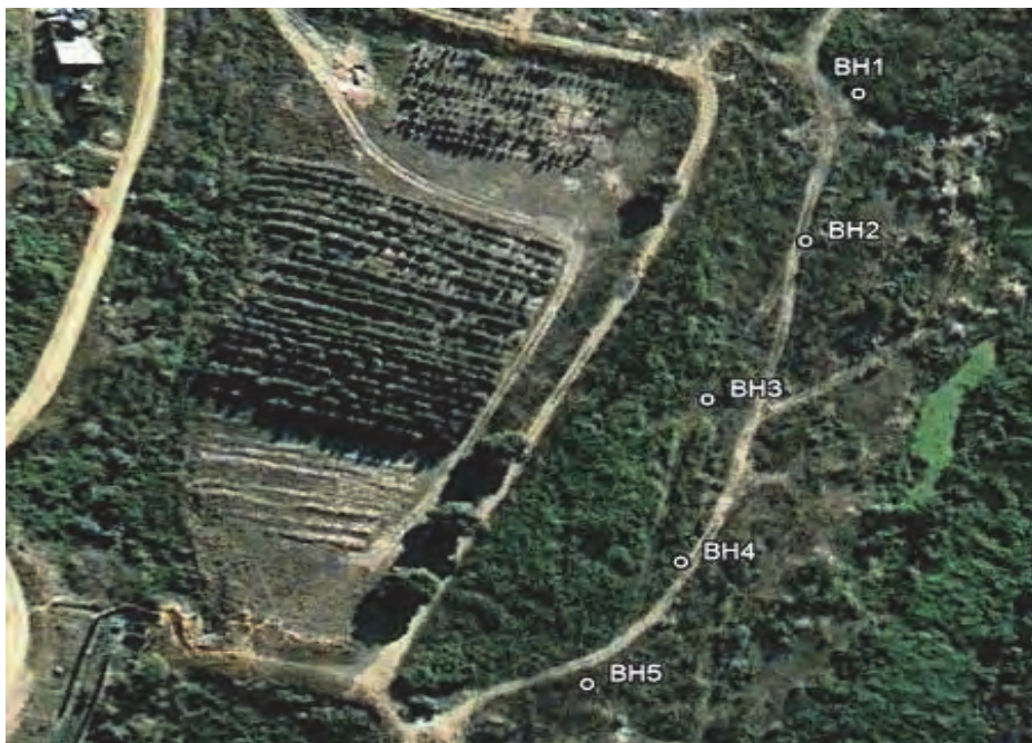
Figure 3.15 Location of borehole sites at Umlazi (BH1 to BH5). The main section of trees was used to monitor changes in sludge composition, the effect on the groundwater and the die off rate of pathogens. Only the nine rows on the northern end of the site were adequately controlled to check the effect on tree growth.
