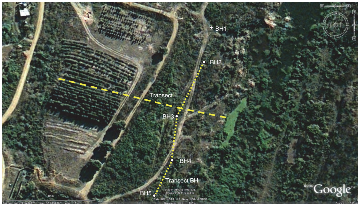
Figure 3.19 Layout of surveyed transects from trench zone to stream and along the borehole line
