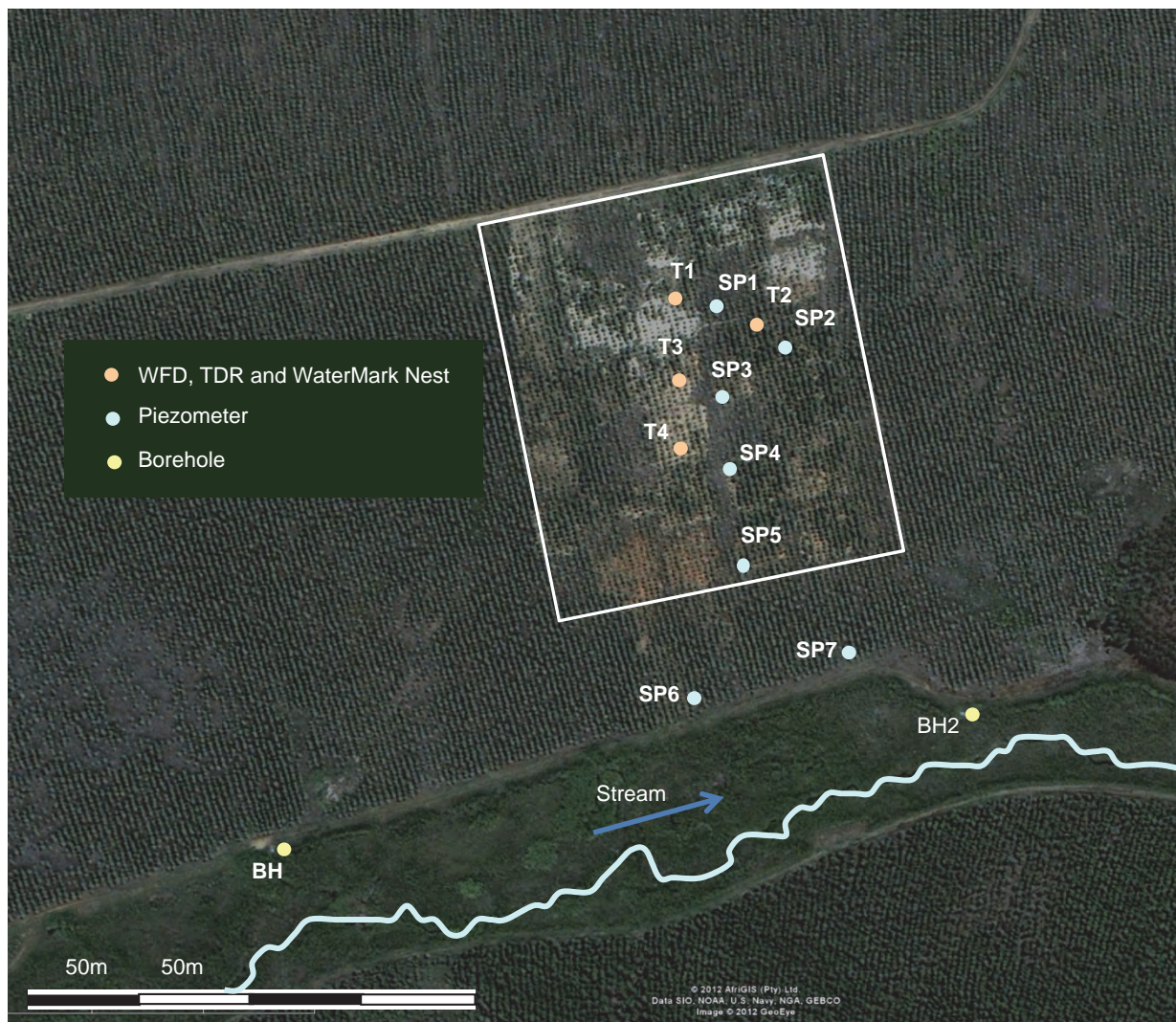
Figure 3.32 Location of groundwater monitoring instrumentation, Sappi site
