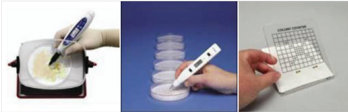
Figure 7-6 Colony Counters: Automatic integrating pen type and Grid plate for manual use
