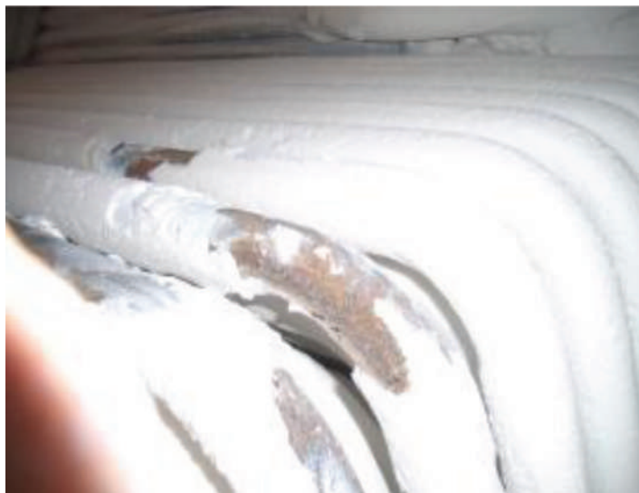
Figure 5.4 Silicon dioxide deposits on boiler tubes
