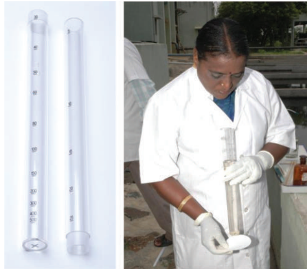
Figure 4.13 Use of a BOD tube for instantaneous assessment of the BOD at site
