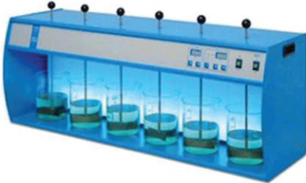
Figure 4.15 Typical Jar Testing apparatus
