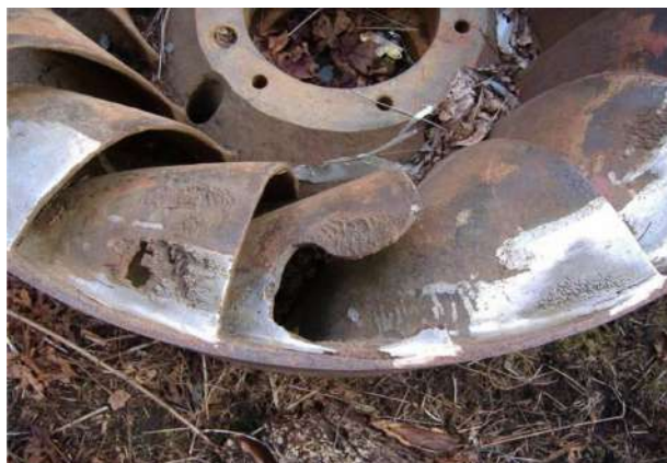
Figure 3.2 Typical Cavitation Damage of an Impeller
