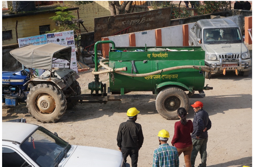
Figure 3. 5 cubic meter pumper truck and tractor owned and operated by a private sector contractor.
