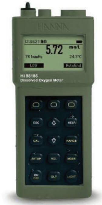
Figure 5-59 Portable BOD test instrument
