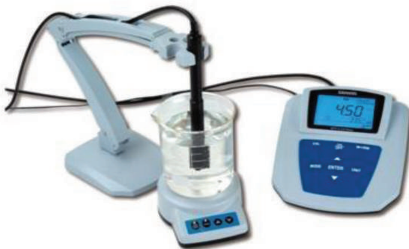
Figure 5-.57 Setup with magnetic mixer and mixed needle for agitation
