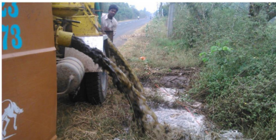
Disposal of septage in open land
