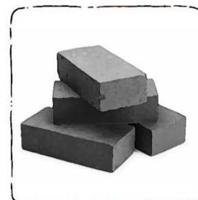
Bricks made from dried fecal sludge
