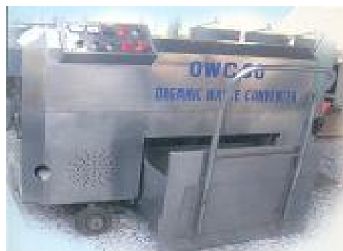
An organic waste converter
