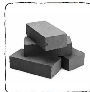
Bricks made from dried fecal sludge
