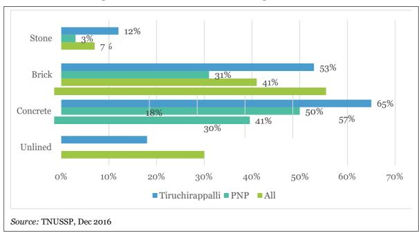
Figure 2.8: Materials Used for Lining Base of the Pit
