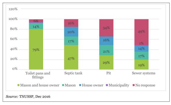
Figure 2.3: Decision Makers for Construction of On-site Systems
