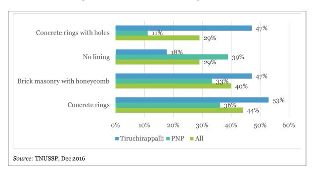
Figure.2.7: Materials Used for Lining Pit Walls
