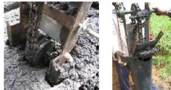
Figure 3.3 Current prototype of Gobbler with single chain and sprung scraper
