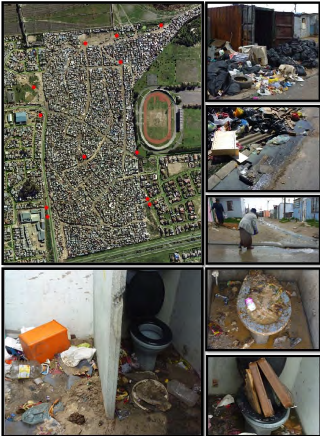
Figure 26: Clockwise from left: (a) solid waste skip locations in Kosovo; (b) a solid waste skip; (c) solid waste and greywater mix together next to a stormwater drain; (d) women dump greywater into a stormwater drain; (e/f) greywater dumped in vacuum toilets; and (g) evidence of open defecation alongside a vacuum toilet (Taing, 14 September, 7 & 9 June 2010).
