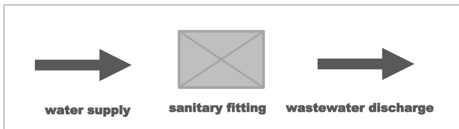
Figure 16: Conceptualising the three areas that can break at each type of sanitary fitting Here the sanitary fitting refers to either the toilets, showers, basins or urinals.
