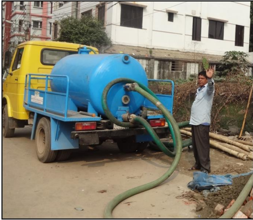
Emptying by vaccum pump (< 100 m sucking pipe) and truck
