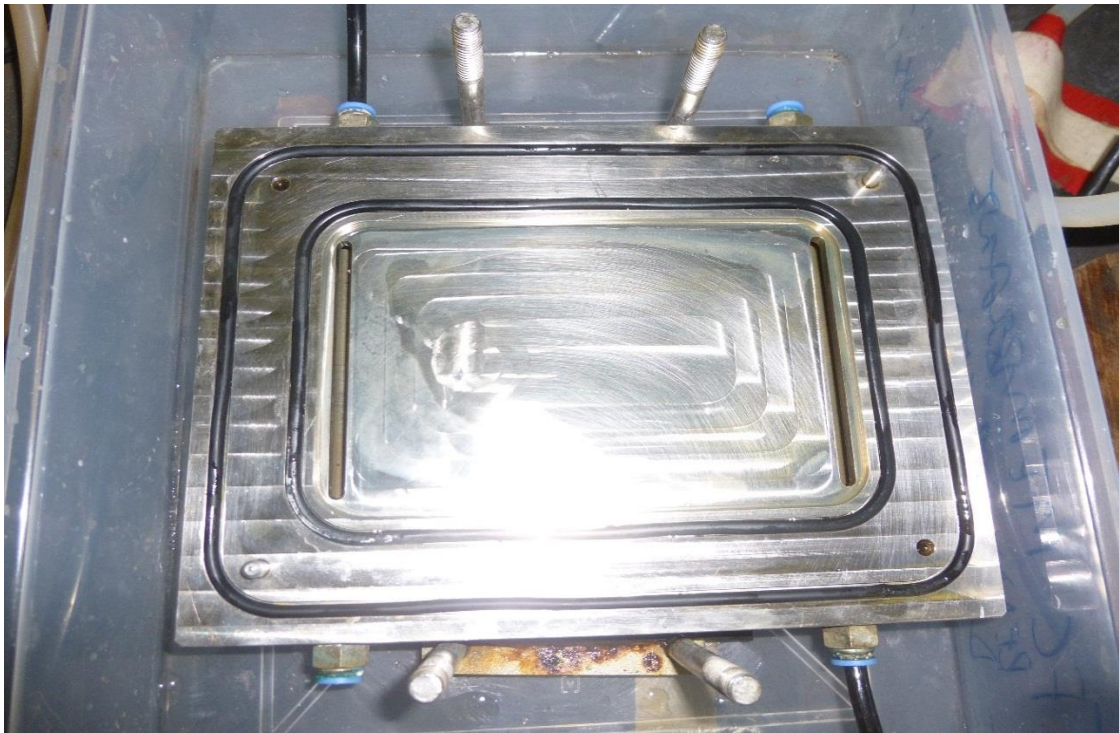
Figure 3-1: Photograph of the FO membrane cell depicting the surface on which the TFC-ES FO membrane sheet is placed. The flow channels of the SEPA cell are also visible on the photograph
