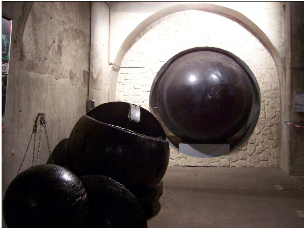
Figure 3: Wooden balls used for cleaning sewers (Flickr, 2009)
