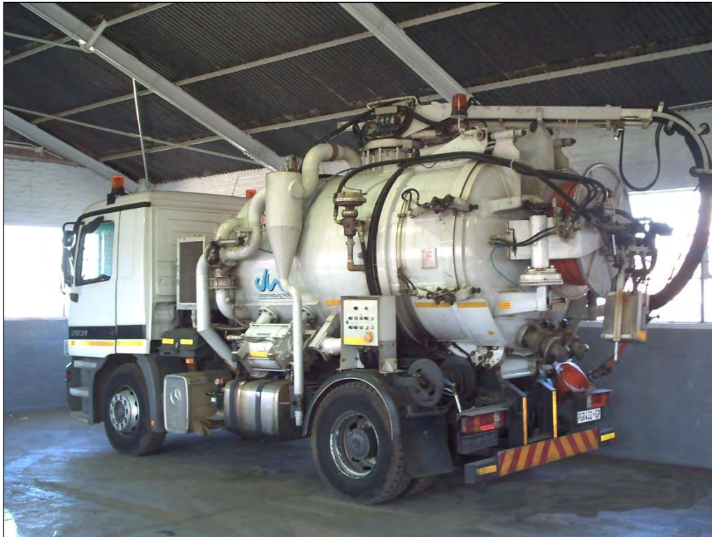
Figure 8: Vacuum and jetting tanker (courtesy of Johannesburg Water)
