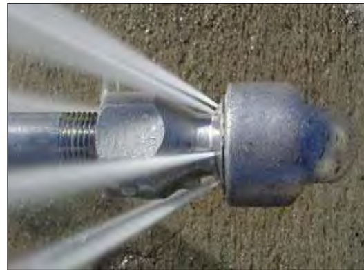
Figure 5: High-pressure nozzle head (Drain Shooter, 2009)
