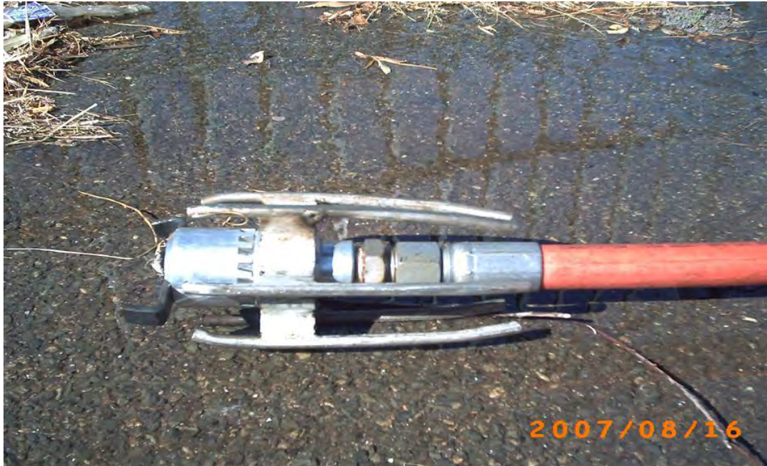
Figure 16: Root cutter (courtesy Johannesburg Water)
