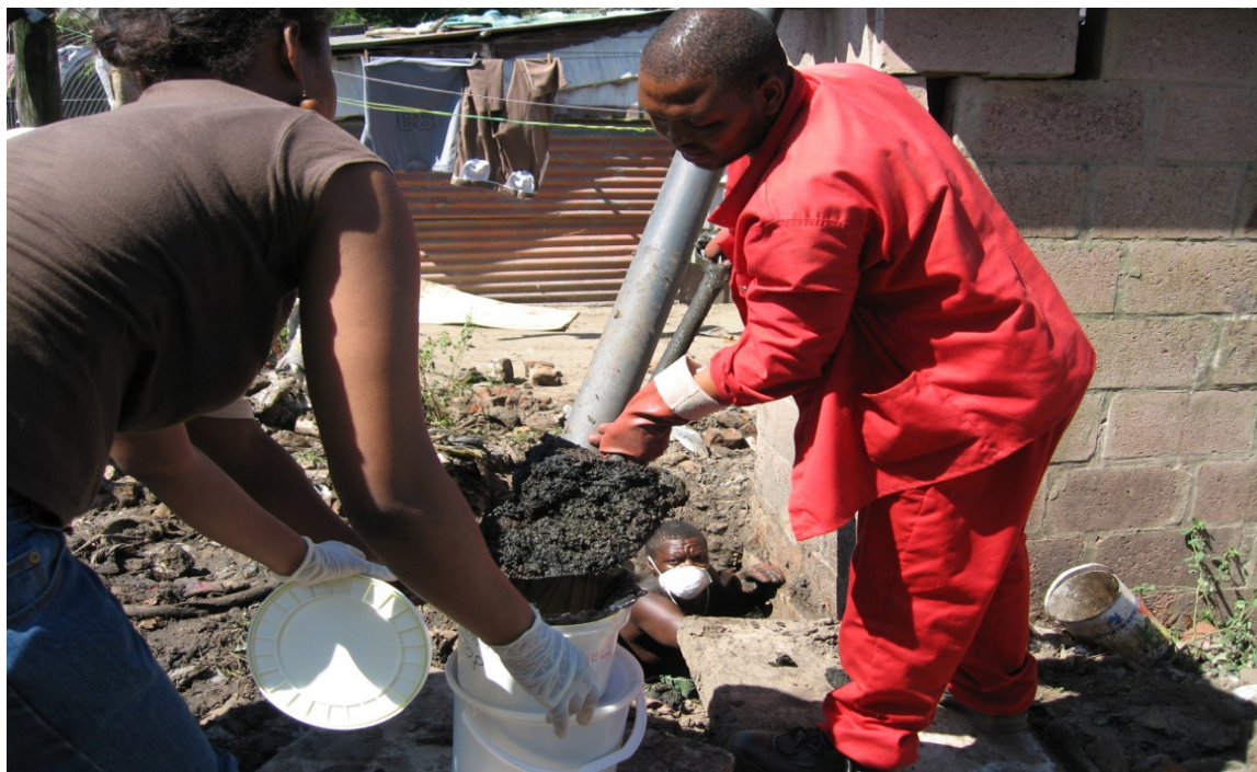
Figure3.1 Photograph showing sampling technique for VIP faecal sludge. Student waiting, to collect contents from different depths within the pit, as emptied by the pit emptier, shown in orange overalls.
