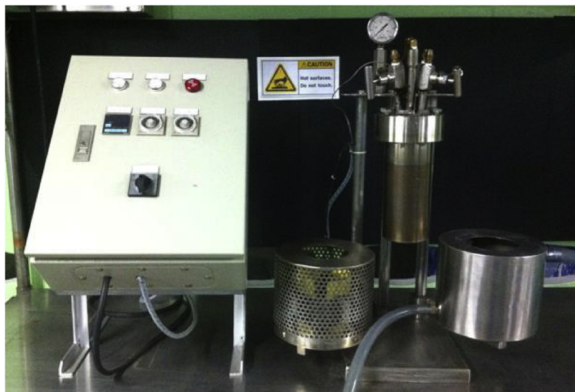
Fig. 1. Photograph of HTC reactor.
