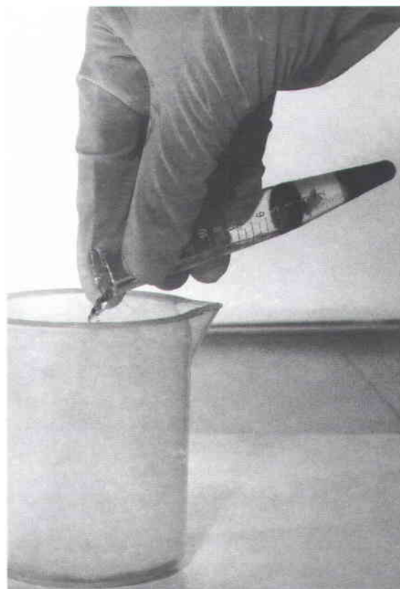
Fig. 7. The supernatant is discarded, leaving only the pellet.
