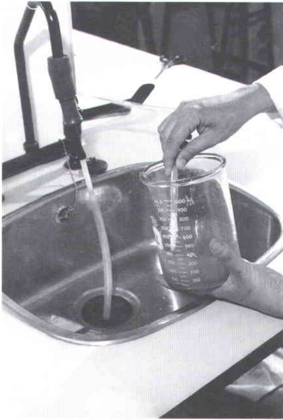
Fig. 2. Removal of the supernatant with a suction pump.
