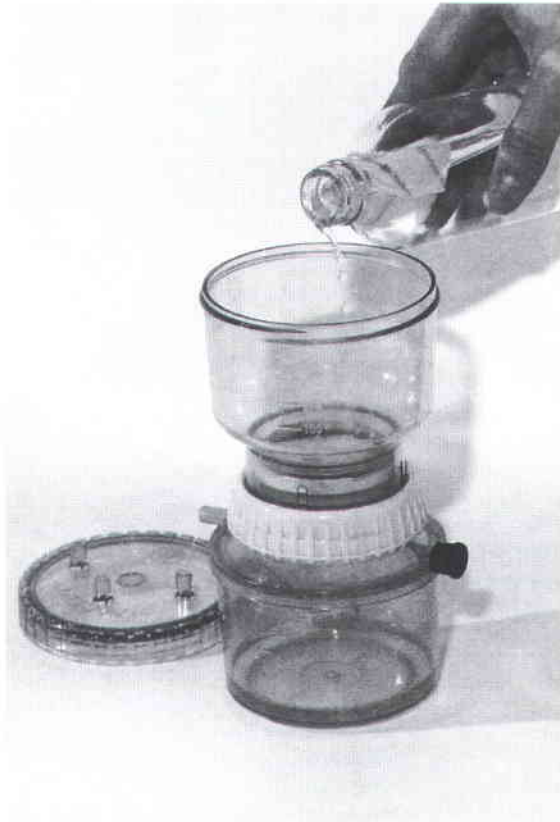
Fig. 19. Pouring about 20 ml of diluent into the membrane filtration unit.
