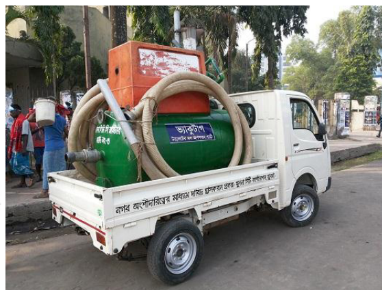
Figure 11 – Retrofitted sludge emptying truck Source: SNV Bangladesh
