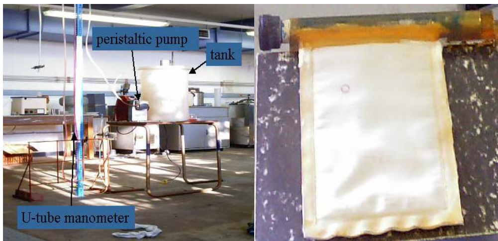
Figure 6-2: The lab scale membrane plant and the fabric membrane used for the tests
