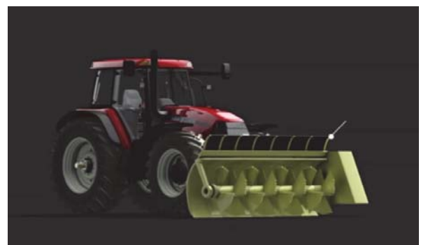
Figure 23: Recent acquisition of tractor-mounted sludge turners with lower capital costs, fuel consumption, local service backup and parts availability.
