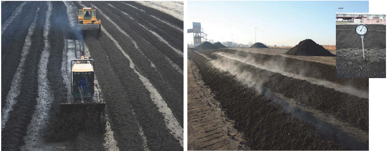
Figure 31: Layout of the windrows and composted sludge at Johannesburg sludge drying and composting plant
