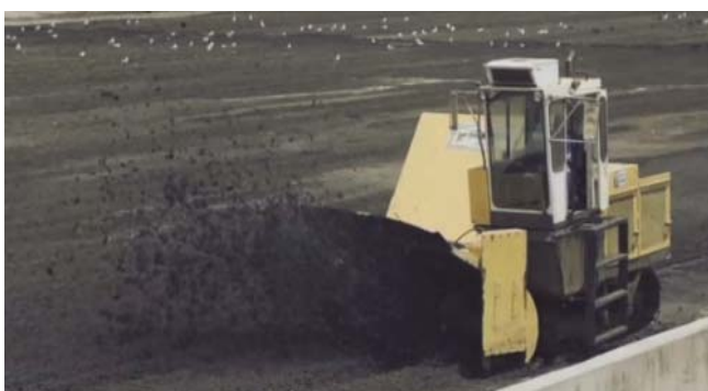
Figure 22: Sludge DS of 70% achieved at NWWTW
