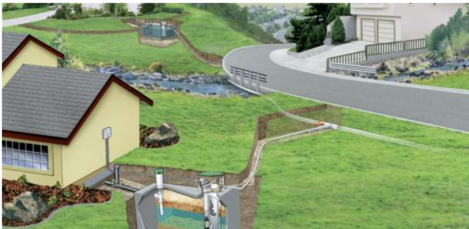
Figure 12: Example of small diameter effluent sewers
