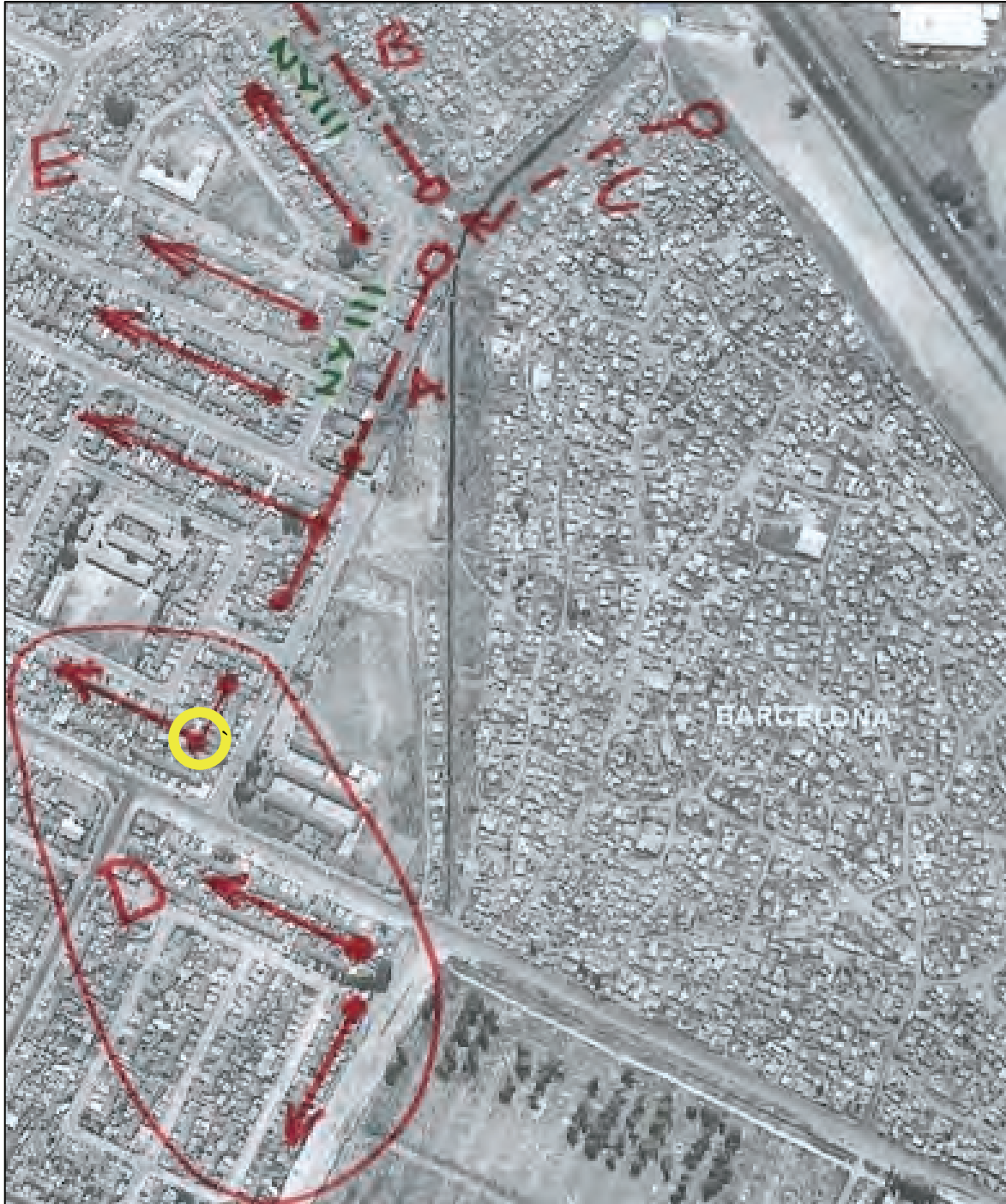
Figure 5-8: The consultant's sketch of the BSSPP's possible sewer connections and routes (BSSPP, 2011). Sections D and E are existing mid-block sewers (one of which was the initial connection highlighted in yellow). The consultant speculated that the pilot could gravitate to the NY 111 sewer (Areas A and B) along a route marked C.
