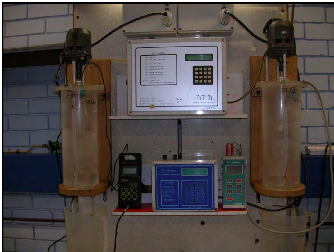
Figure 51 Batch reactors set up for aerobic batch tests.
