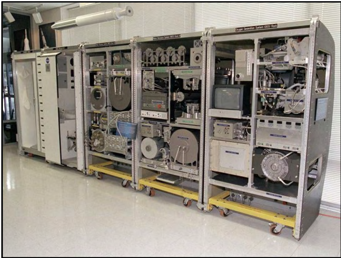
Figure 8 Treatment plant installed in the International Space Station for the complete recovery of fresh water from urine 3
