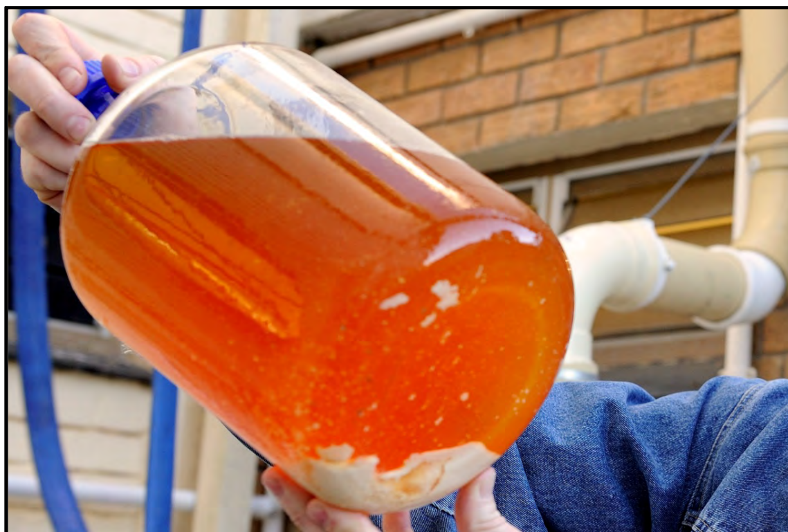
Figure 20 Schott bottle filled with stored urine and precipitated salts on the bottom.
