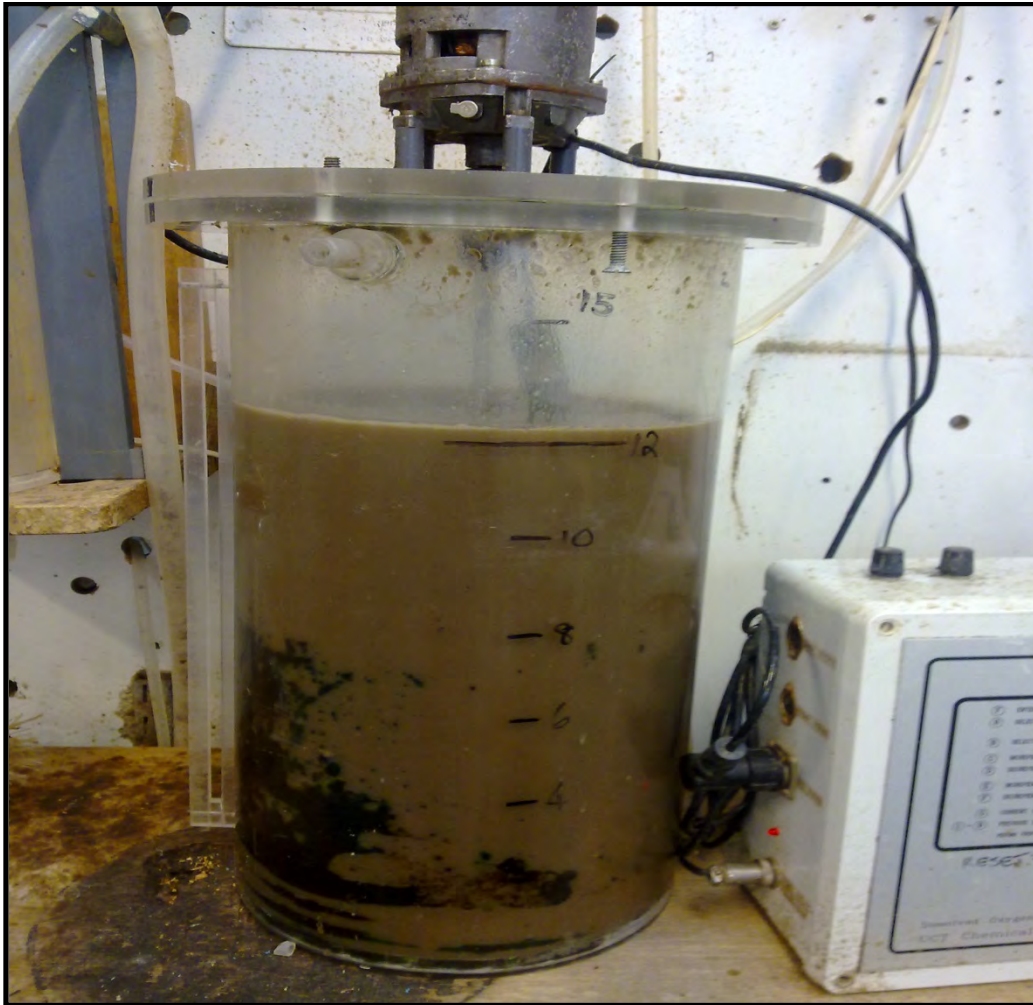
Figure 40 Anoxic-aerobic digester, with stirrer, air pipes and OUR recorder
