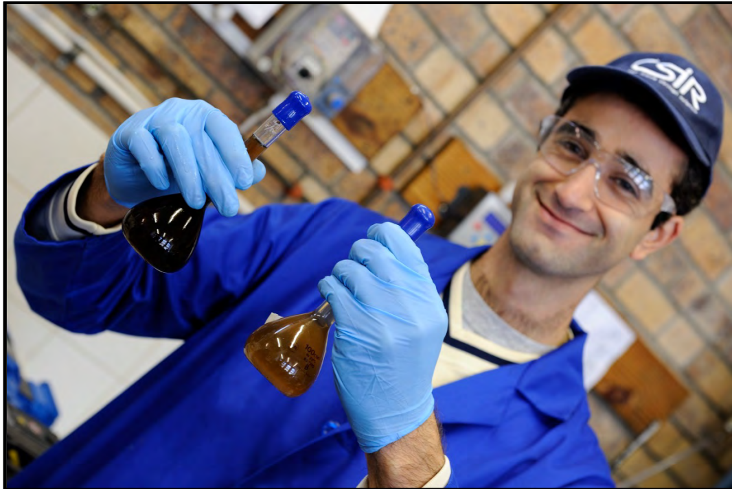
Figure 5 Two samples of urine; on the left is undiluted stored urine from men's urinals while on the right is urine treated in the sequencing batch reactor
