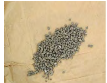
Figure 1: Latrine Dehydration Pasteurization (LaDePa) agricultural pellets processed from sludge.
