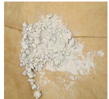
Figure 1: Struvite processed from source-separated urine
