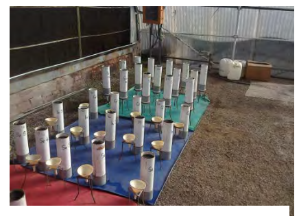
Figure 2: N and P retention investigated in a column experiment
