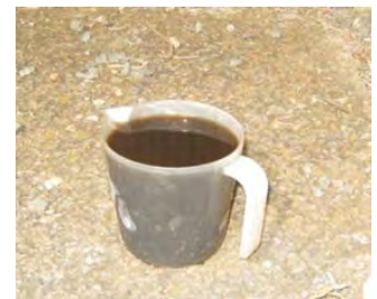
Figure 2: Nitrified Urine Concentrate (NUC) processed from source-separated urine
