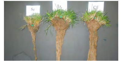
Figure 3: Perennial root growth in the Sepane (Se), Inanda (Ia) and Cartreff soils (Cf) in columns irrigated using DEWATS effluent
