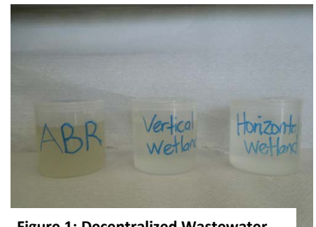
Figure 1: Decentralized Wastewater Treatment (DEWATS) plant effluent
