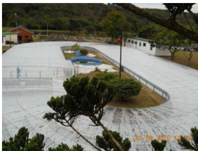
Algae being cultivated in the 300 000 L raceway pond at Kingsburgh wastewater treatment works
