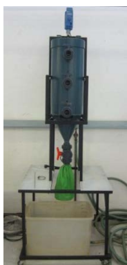
Figure 1: Struvite reactor at UKZN (left); Nitrification reactor at Eawag (middle); Evaporation reactor (right, © KMU Umweltschutz GmbH)
