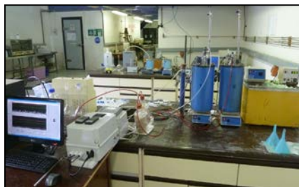
Anaerobic Batch stirred Reactors (ASBR's) located at the Pollution Research Group laboratories
