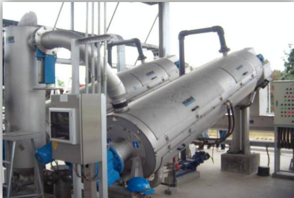
Screw Press for de-watering/ separation of sludge and filtrate
