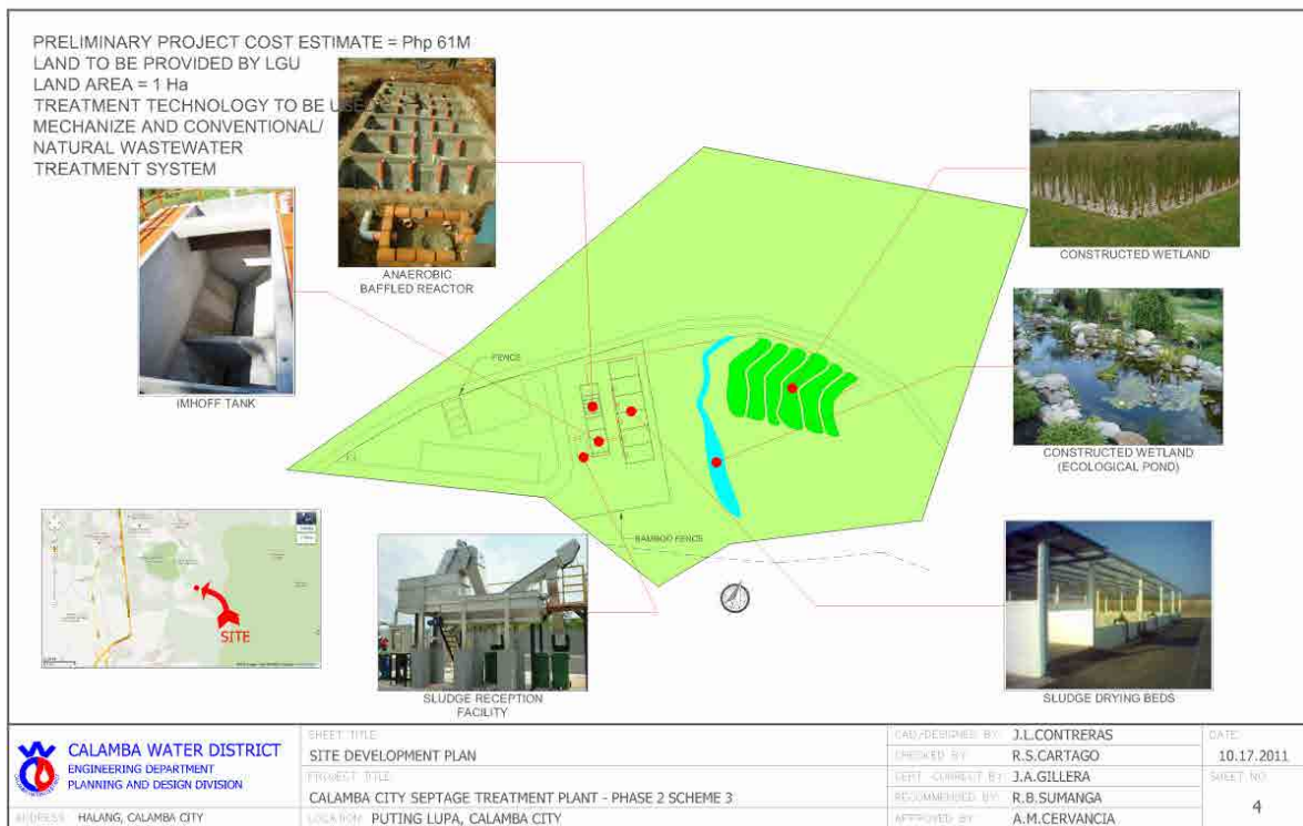
Figure-6.4.2 Layout of Treatment Facilities
