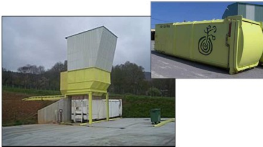
Figure 3: Left: Transfer Station for Solid Waste (Container with compaction unit underneath the hopper). Right: closed container.
