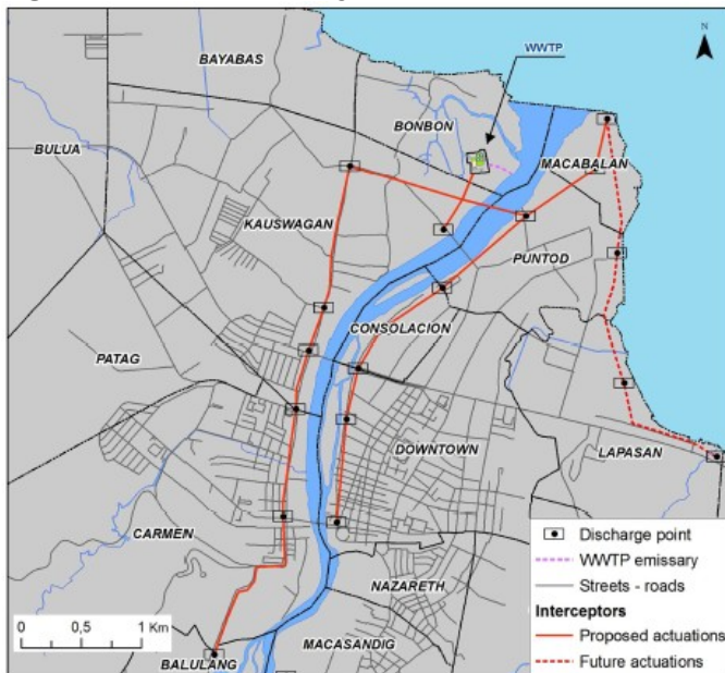
Figure 5: Interceptor System in CdeO
