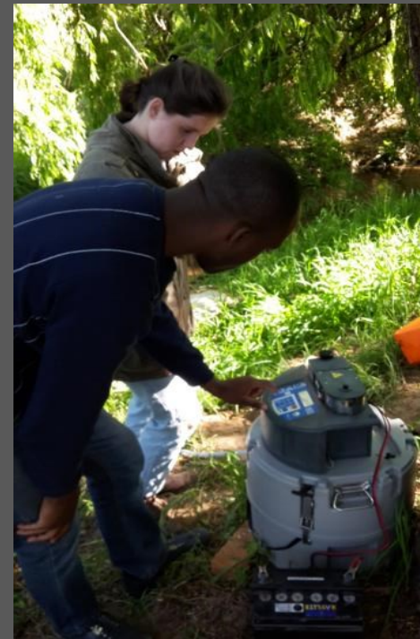
Discrete water sampling using an auto-sampler
