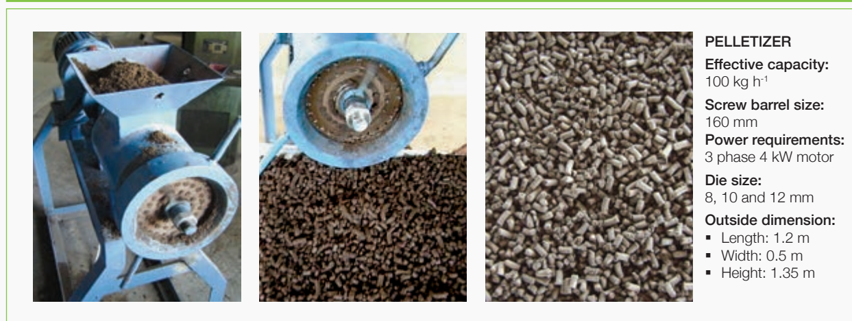
FIGURE 23. PELLET PRODUCTION – A) PELLETIZER BEING OPERATED, B) NEWLY PRODUCED PELLETS, AND C) FINAL PELLETS (AFTER DRYING AND SIEVING).
