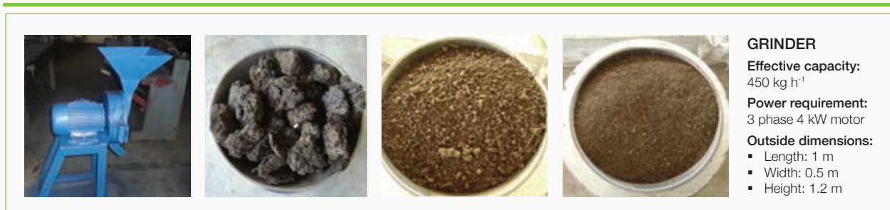
FIGURE 21. A) THE GRINDER, B) RAW DFS, C) C-DFS NOT GROUND, AND D) GROUND C-DFS.
