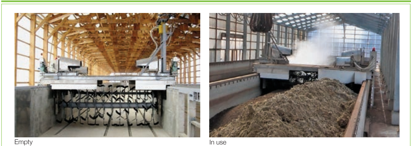
FIGURE A8.2.1. THE HOSOYA SYSTEM APPLIED IN GREECE AND THE UNITED STATES.
