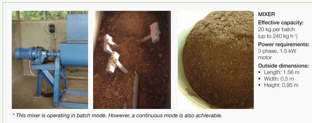
FIGURE 22. DFS COMPOST ENRICHMENT-MIXER (A) SIDE, (B) TOP VIEWS, AND (C) NEWLY PRODUCED ENRICHED DFS COMPOST.
