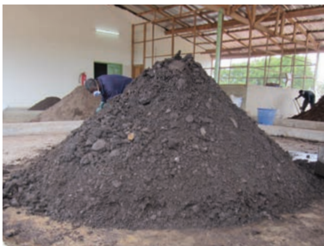
FIGURE 16. HEAP COMPOSTING OF DEWATERED FS.
